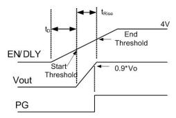
Figure 2. Soft-start Timing Diagram
