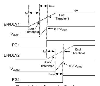
Figure 4. Output Sequencing Waveforms
