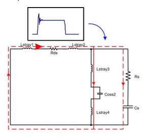
Figure 11. Snubber Circuit
