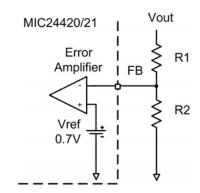
Figure 8. Setting the Output Voltage
