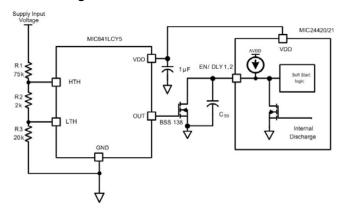
Figure 1A. Adjustable UVLO startup circuit
