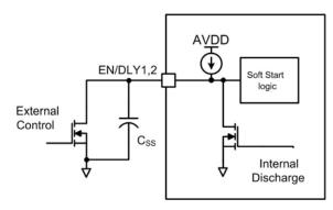
Figure 1. Enable and soft-start circuit
