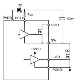
Figure 5. High-side Drive Circuitry
