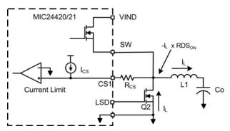
Figure 7. Over-current Circuit
