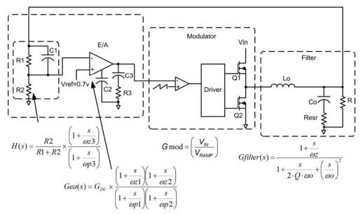
Figure 12. Voltage Loop and Transfer Functions
