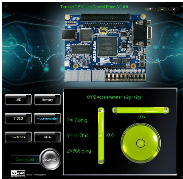
Figure 2-7 Level by G-Sensor
