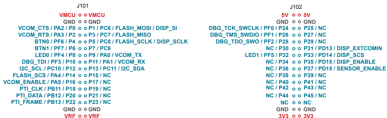
Figure 4.2. Radio Board Pin Mapping on Breakout Pads
